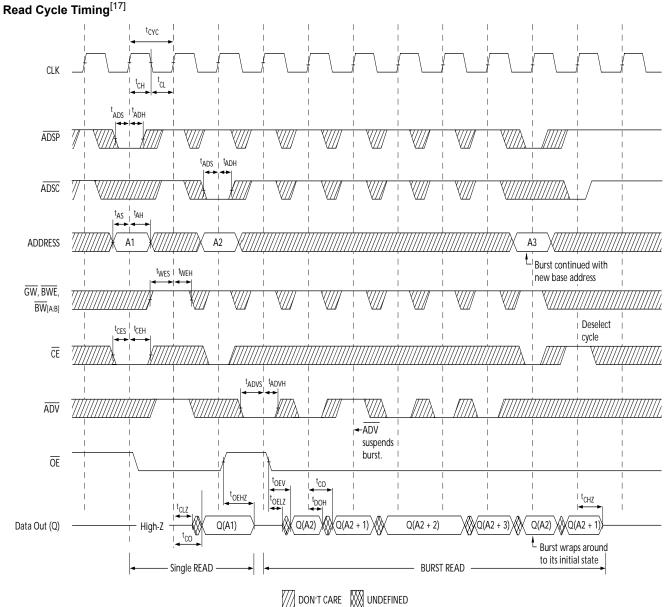
**Note:** 17. On this diagram, when  $\overline{CE}$  is LOW,  $\overline{CE}_1$  is LOW,  $CE_2$  is HIGH and  $\overline{CE}_3$  is LOW. When  $\overline{CE}$  is HIGH,  $\overline{CE}_1$  is HIGH or  $CE_2$  is LOW or  $\overline{CE}_3$  is HIGH.
