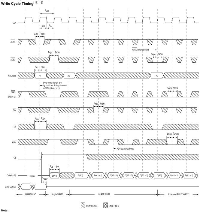
18. Full width Write can be initiated by either  $\overline{\text{GW}}$  LOW; or by  $\overline{\text{GW}}$  HIGH,  $\overline{\text{BWE}}$  LOW and  $\overline{\text{BW}}_{[A:B]}$  LOW.
